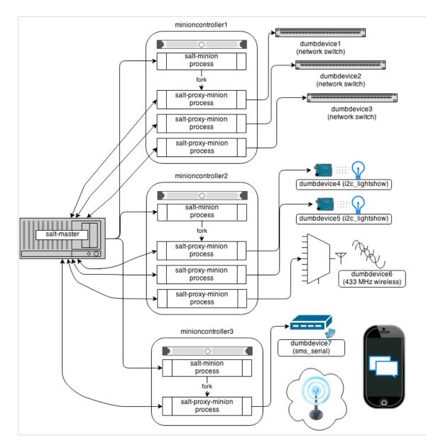
The key thing to remember is the left-most section of the diagram. Salt's nature is to have a minion connect to a master, then the master may control the minion. However, for proxy minions, the target device cannot run a minion, and thus must rely on a separate minion to fire up the proxy-minion and make the initial and persistent connection.
