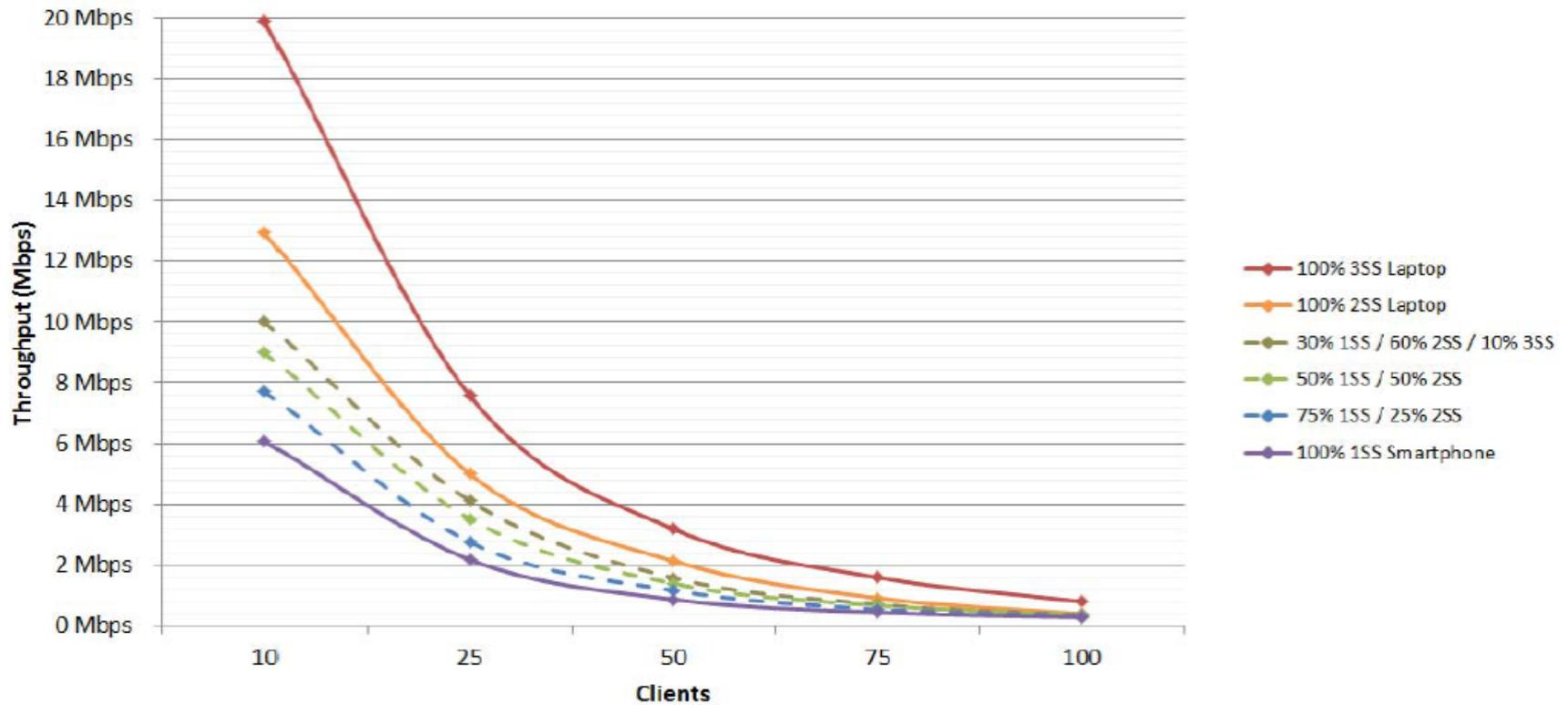
**Figure T4-10** Average Per-Device Throughput (AP-225, VHT20, TCP Bidirectional)
